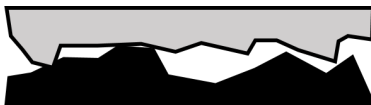
Figure 5.3: Illustration that the frictional force between surfaces can be thought of as arising from microscopic imperfection in the surfaces, although even two perfectly smooth surfaces would still interact.
