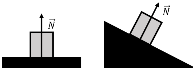
Figure 5.2: The normal force, \vec{N} , exerted by a horizontal surface on a block (left side) and by an inclined surface (right side). In both cases, the normal force on the object is perpendicular to the interface between the object and the surface and points in the direction from the interface towards the object.
