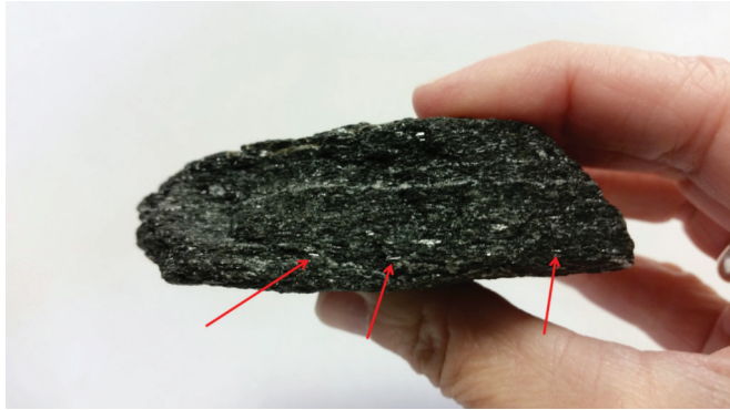
Figure 11.4 | Example of a foliated amphibolite. Notice the alignment of the amphibole minerals, best seen where the red arrows are indicating. The lighter colored minerals in this rock are plagioclase feldspars.
