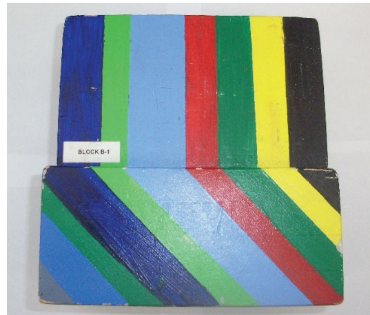
Figure 12.5 | You are viewing the top block in this image in map view, viewed from directly above the block. The lower block is from the same rock layers, and you are viewing it in cross-section (or from the side). Note that in cross-section, you can see how the rock layers are tilted.
