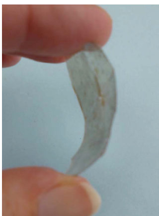
Figure 7.19 | Muscovite mica, which bends but returns to its original shape, is elastic.
