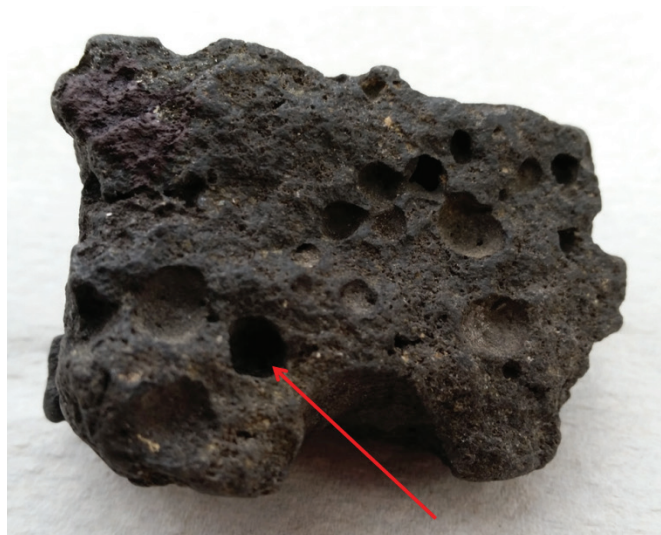
Figure 8.8 | An aphanitic mafic rock (basalt), with gas escape structures called vesicles. Arrow points to one vesicle that is ~1cm in diameter. This is an example of another texture type, called vesicular texture, and the name of this rock is a vesicular basalt.
