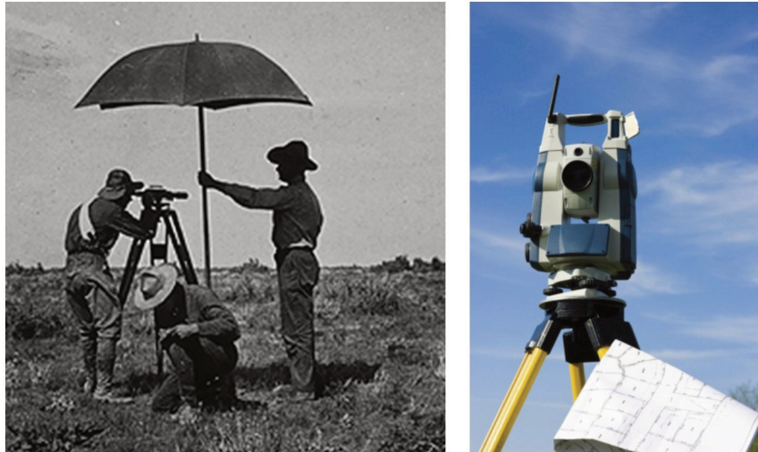
Land surveying. The foundation for modern mapping was laid by people walking and measuring the land with specialized telescopes (left) and modern GPS enabled total stations (right). 23
