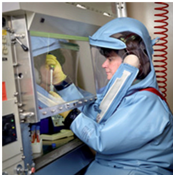
Figure 9.2 A protective suit like this one is an additional precaution for those who work in BSL-4 laboratories. This suit has its own air supply and maintains a positive pressure relative to the outside, so that if a leak occurs, air will flow out of the suit, not into it from the laboratory. (credit: modification of work by Centers for Disease Control and Prevention)
