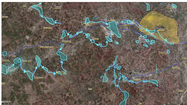
Figure 54 Interconnected ponds overflow from one to the next between multiple villages within a watershed.
