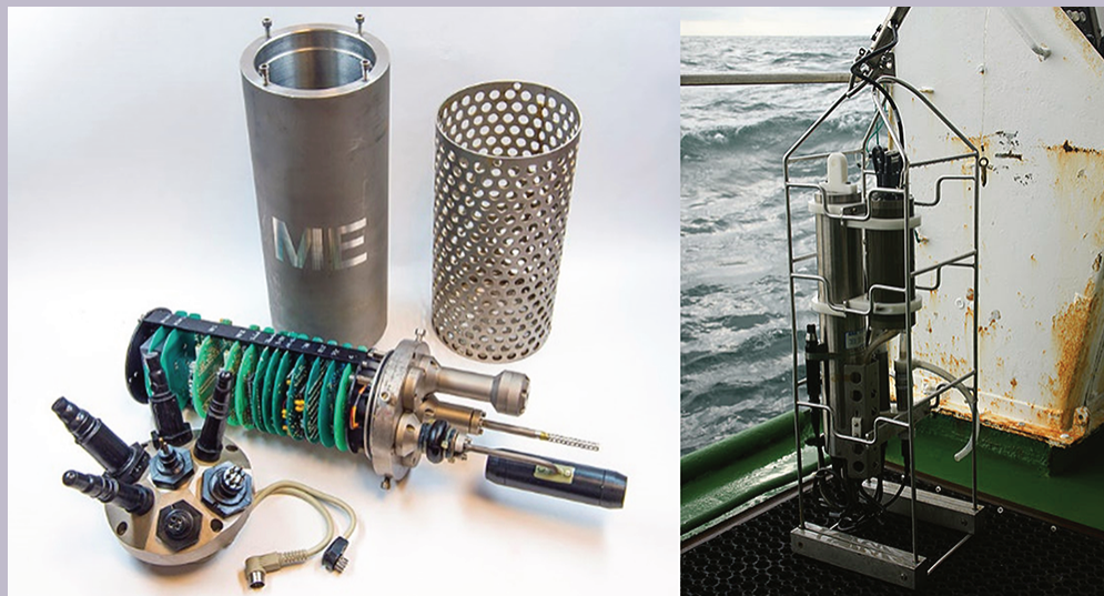
Left: The inner workings of a CTD. An array of different probes are attached. Right: A CTD in a protective cage ready to be deployed at sea. (Left: Hannes Grobe [CC BY 3.0 ( https://creativecommons.org/licenses/by/3.0/ )]; Right: © Hans Hillewaert (CC BY-SA 4.0) via Wikimedia Commons)
