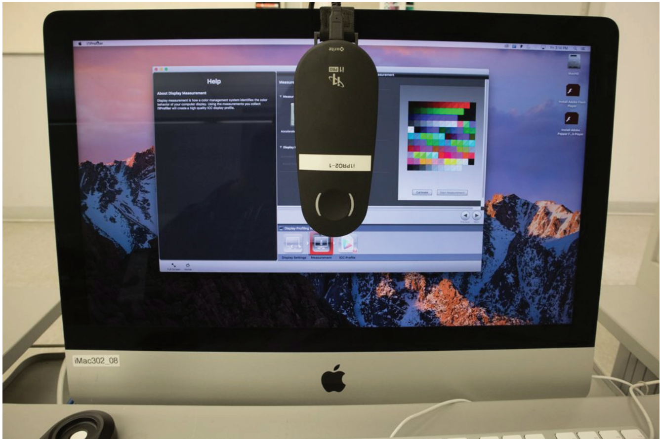
Figure 4-11. A monitor profile being made with an X-Rite i1 Pro 2 emissive/reflective instrument and i1 Profiler software.
