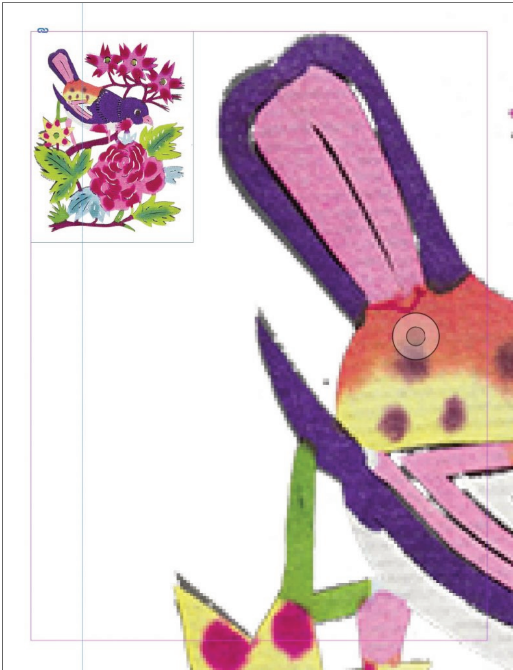
Figure 3-2. The image on the left has been placed at 100% of size, and has a resolution that is appropriate for printing. The image on the right has been enlarged 800%, effectively lowering the resolution, resulting in a pixelated image.
