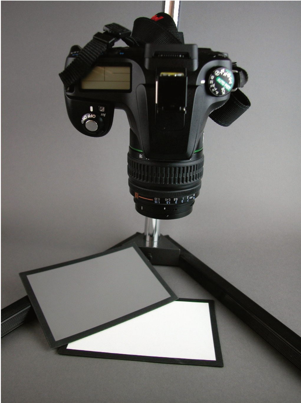
Figure 2-11. A copy stand is useful for photographing flat subjects. This photo also shows an 18% gray card, useful for setting exposure to 0 EV, and a white card, used for setting white balance. (White balance can be set on either the gray or white cards, provided that both are colorimetrically neutral.)
