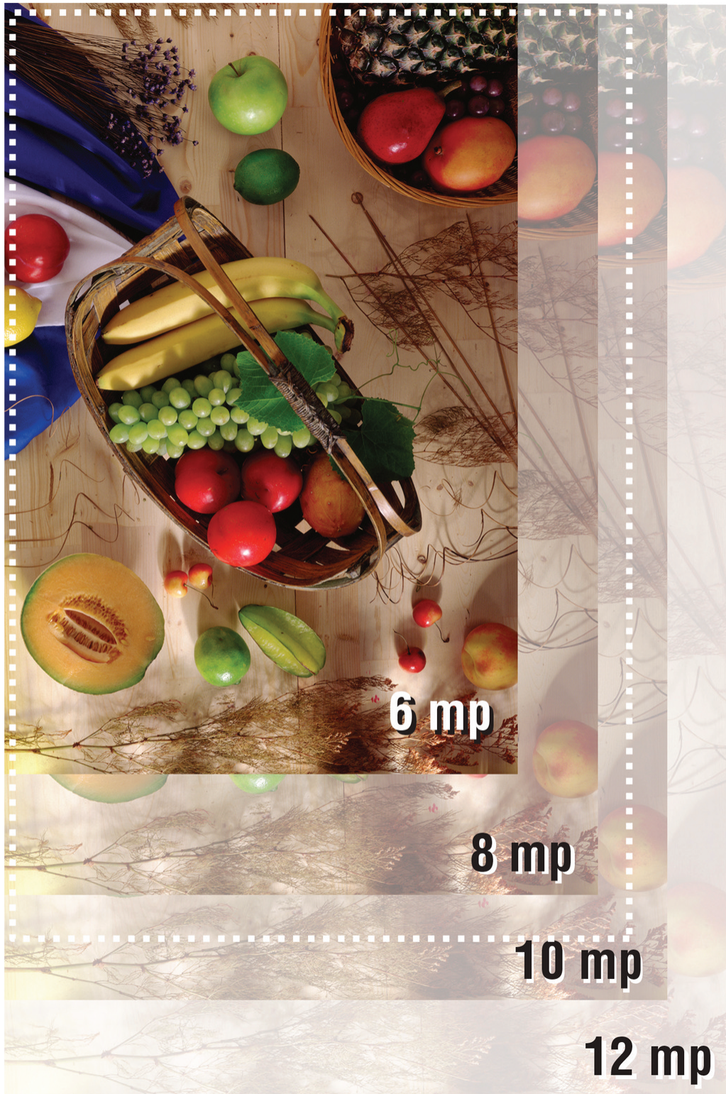
Figure 2-3. Printed images require sufficient megapixels to support their resolution and screening. This diagram shows the relative sizes of various megapixel images in relation to an 8.5×11-in. page (white dotted outline), which requires 8.5 MP for full coverage.
