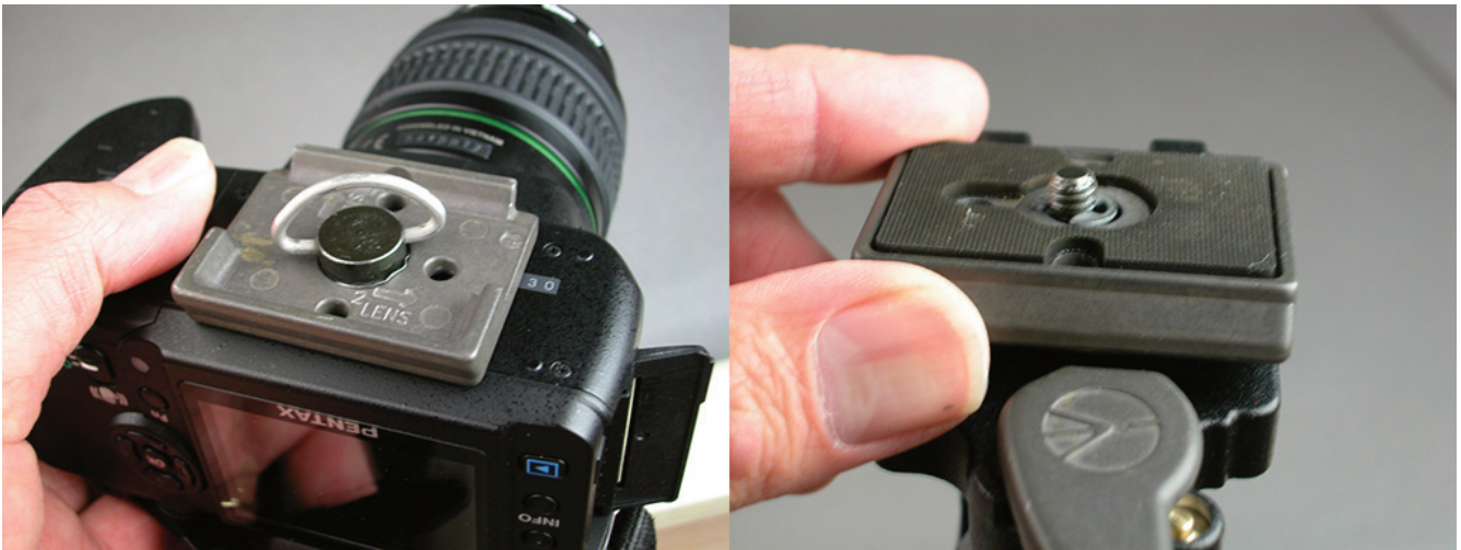
Figure 2-10. Camera attachments. A quick-release tripod mount has a detachable bracket that is screwed into the camera's tripod mount and then clamped to the tripod.
