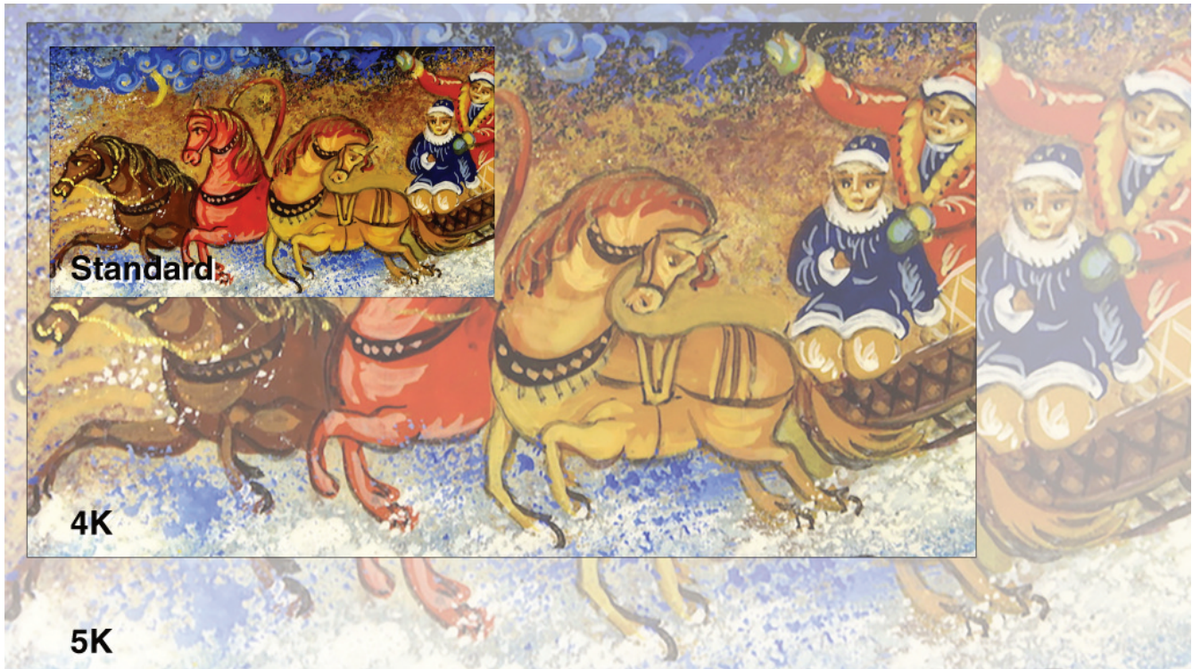
Figure 2-4. Relative sizes of images for the web on standard (1920×1080 21-in.), 4K (4096×2304, 21-in.), and 5K (5120×2880, 27-in.) displays (compare with Table 2-1).
