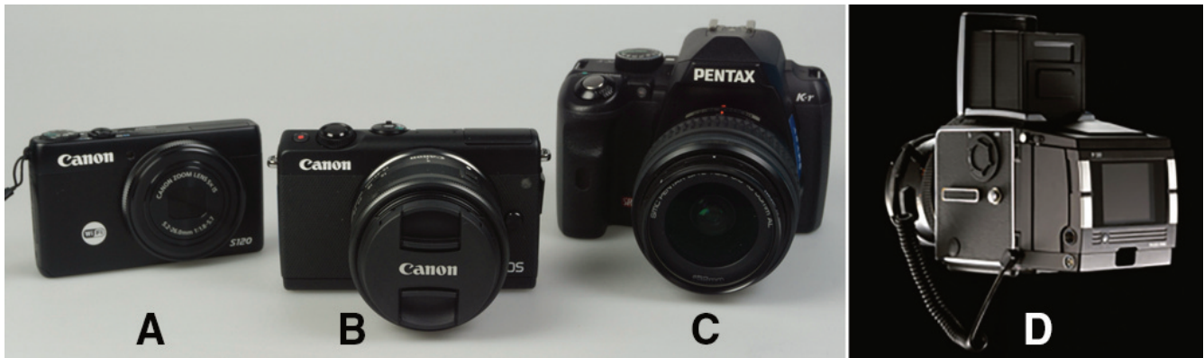
Figure 2-1. Camera systems. A. A Canon S120 (12MP) professional point-and-shoot camera with fixed lens. B. A Canon EOS M100 mirrorless camera (24MP) with removable lenses. C. A Pentax K-r DSLR (16 MP), D. A Hasselblad professional medium-format camera with a digital back (40MP).
