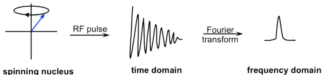
Figure 6.5d Simplified diagrams to illustrate NMR experiment
