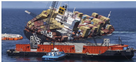
Fig. 1.4 – Containers falling from a their location on a ship after rolling rotation.
